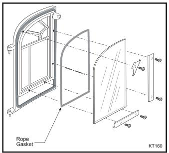
Fig. 28 Door glass installation.
